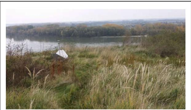
Fig. 3. View of a single reflector benchmark with the GNSS adapter emplaced on the subsiding loess bank, near the settlement of Dunaszekcső with the River Danube in the background.
