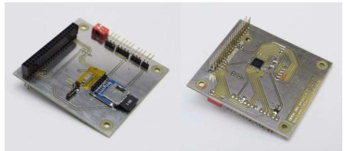
Fig. 2 On-Board Computer Flight Model
