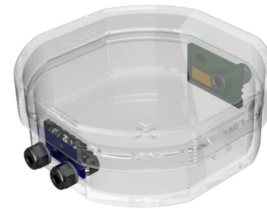
Fig. 4. Custom design of a petri dish with sensor adaptation
