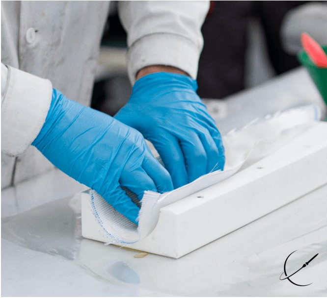
Fig. 1.: Gaining practical knowledge is important when working in a team. The picture shows the production of one of the rocket bodies. The team's knowledge of polymer technology is outstanding.
