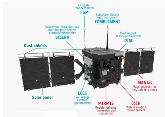
Figure 3. Scientific instruments positions on the main probe A
