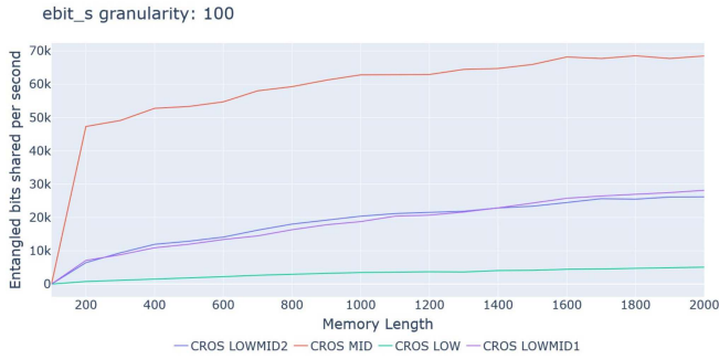
Figure 5. Plot for the CROS constellations average share entangled quantum bits per second with granularity set to 100.
