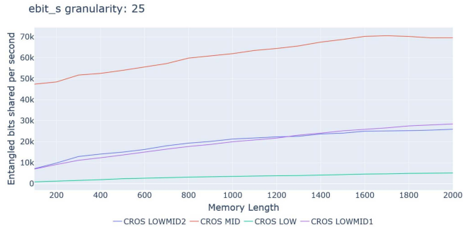
Figure 6. Plot for the CROS constellations average share entangled quantum bits per second with granularity set to 25.
