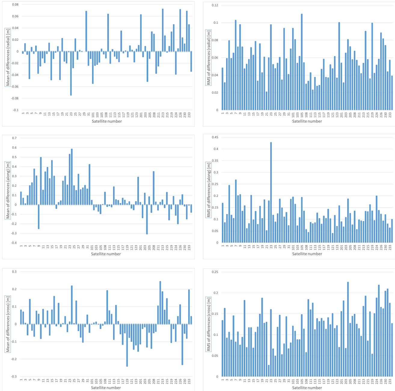
Fig. 7. Mean and root mean square (RMS) of differences for each satellites. Satellite number 1-99 are GPS, 101-199 are GLONASS and 201-299 are Galileo
