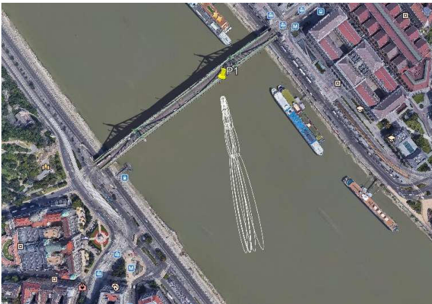
Fig.5 The Fresnel-zones of the GPS satellite G28 for the DOY 037 (2020).
