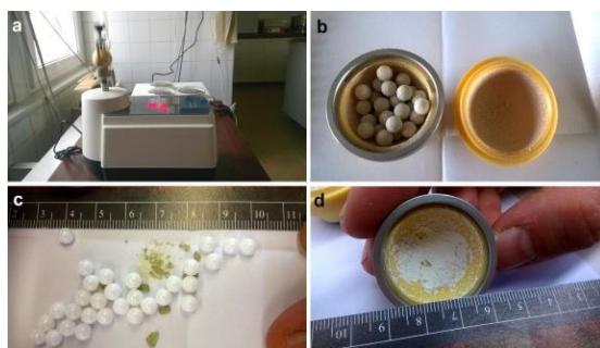
Figure 1. Images related to the pulverizing capability. a: the pulverizer during vibration (the sample is inside the zirconium-oxide sphere at the top left), b: the interior of the mortar with the zirconium-oxide balls, c: balls with weakly pulverized olivine grains (fragments are green and mm sized), d: fine powder produced by long duration (several minutes) pulverizing.
